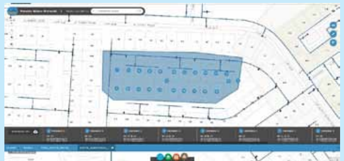
Example 2 of GIS tools: Isolation Trace tool in PW. This tool allows the user to allocate pipe break location and identify all isolation valves and affected customers. It also gives the option to download, print or send the information or map to operation or maintenance teams to take the required actions.
