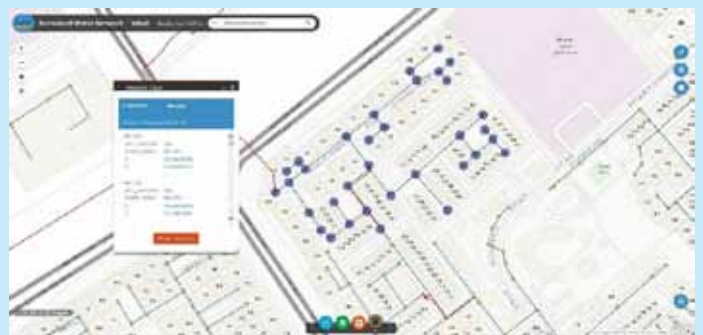
Example 1 of GIS tool: Manhole Trace tool in RW. This tool identifies all manholes related to a specific Lift Station and gives the option to download, print or send the information or the map to an operation team for flushing or other purposes.
